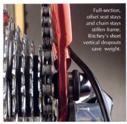
the Thunder and Storm are built with stouter tubing and longer chainstays. The bottom bracket is kicked up for single-track boulder-hopping.
